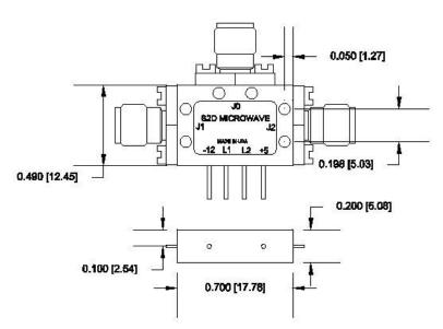
Ground and Bias connector - solder pins
